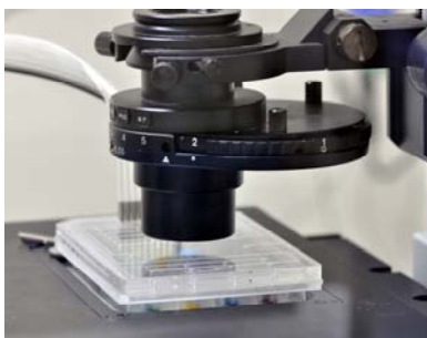
Figure 3. Manifold Sealed to Plate on Microscope Stage
