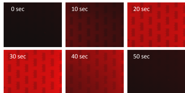
Solution exchange profile at 2 psi between a fluorescent dye and buffer solution in a 0.25x0.2 mm field of view (20X objective).
